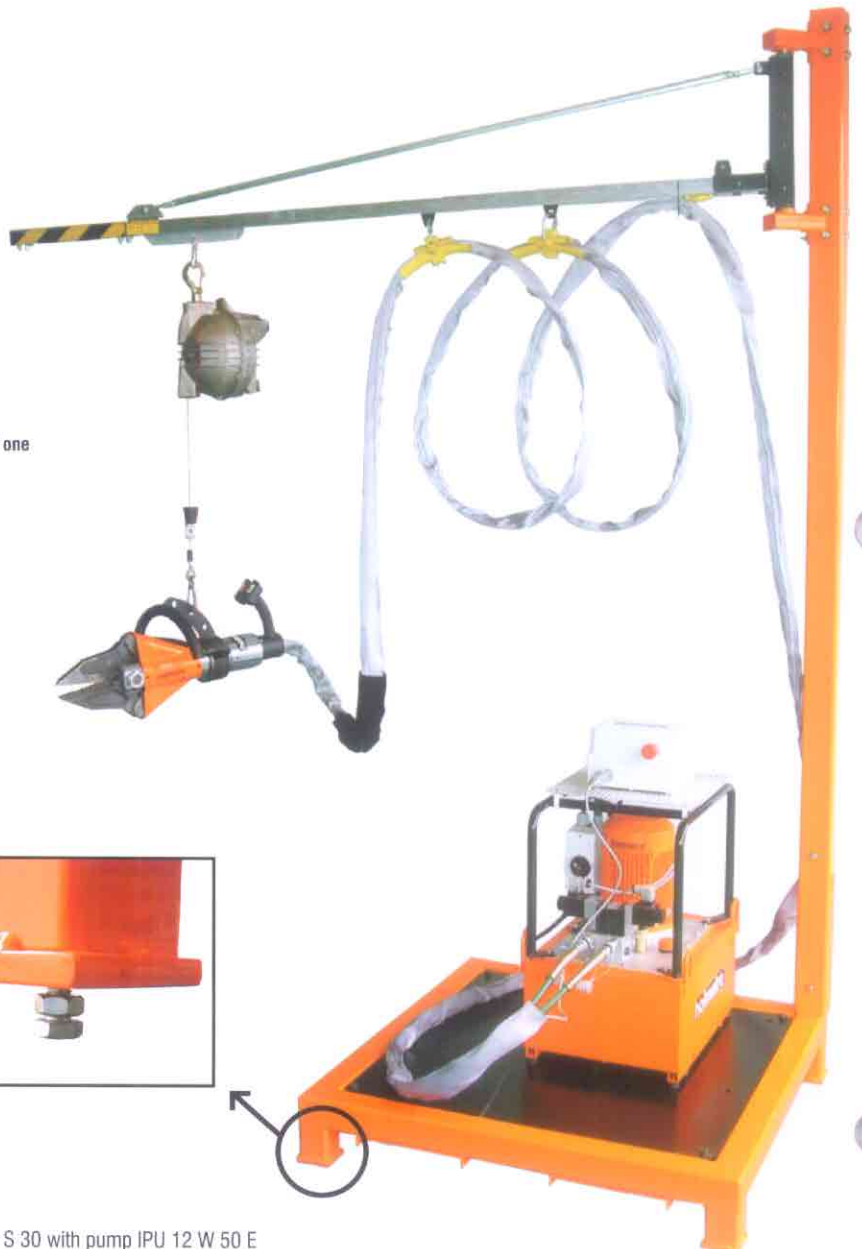
2035 DU pump with mobile cutter ICU 10 A 40
